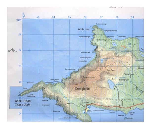
The grid is made up of the Eastings (Vertical lines) and the Northings (Horizontal lines)
