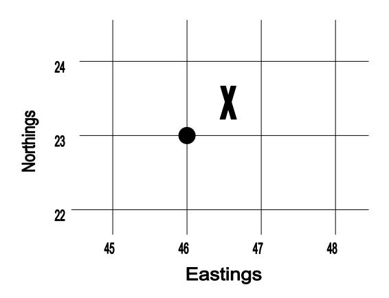
To give a 4 figure grid reference of the marked square we give the numbers of the two lines that cross at the bottom left of the square.
