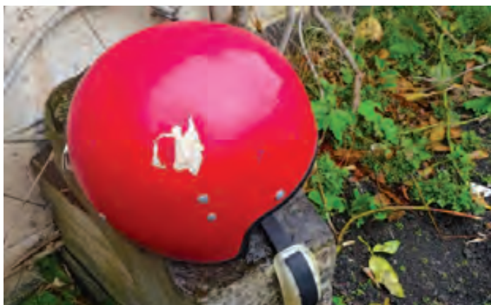
Old-style helmet that sustained a severe blow in a climbing accident
